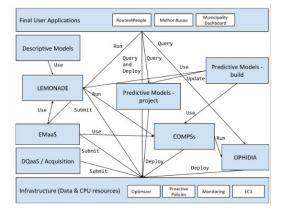
Figure 4. The software architecture for the three applications.
