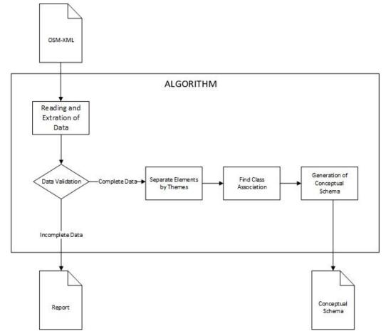
Figure 3. Simplified flowchart of the method proposed for generating the conceptual database schema
