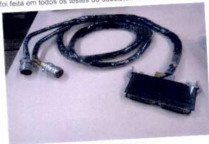
Figura 2 – Slot Feed-Thrus
