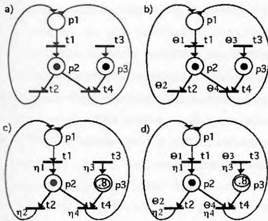
Fig 1- Examples of Petri net formalisms ( $\theta_i = \theta(t_i)$ ,  $\eta_i = \eta(t_i)$ ),
