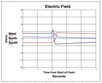
Figure 14. Ambient electric field meter recordings for an upward flash with an UPL. The red trace is from the West Sensor site EFM, the black trace is from the North Sensor site EFM, and the blue trace is from the South Sensor site EFM.
