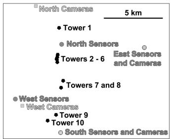
Figure 2. Layout of the 10 towers relative to the electric field sensing instrumentation and cameras.
