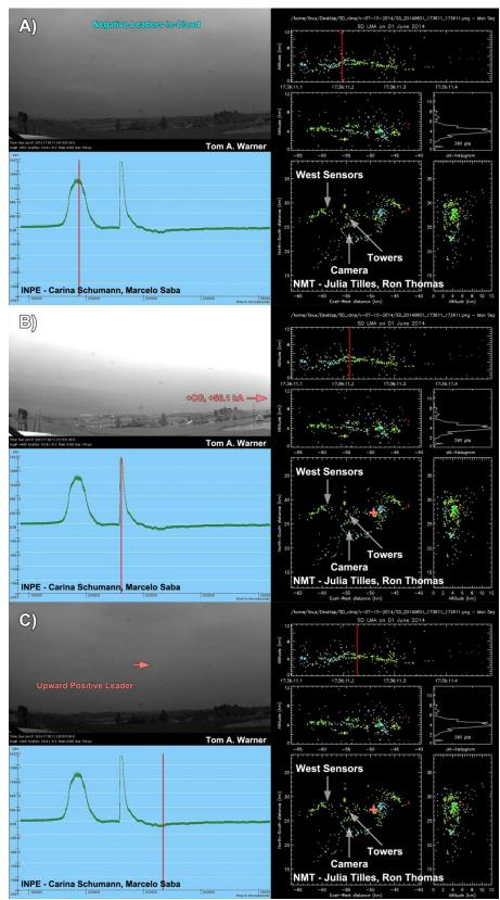
Figure 9. Composite figure showing images from a high-speed video recording (upper left panel), electric field change sensor recording (lower left panel) and LMA display (right panel). Red vertical lines show correlated time with high-speed video image.
