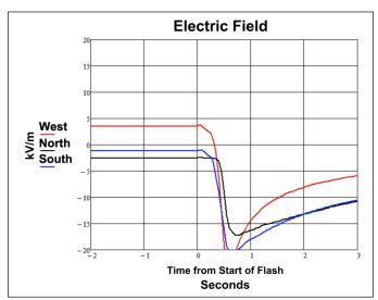
Figure 15. Ambient electric field meter recordings for an upward flash with an UNL. The red trace is from the West Sensor site EFM, the black trace is from the North Sensor site EFM, and the blue trace is from the South Sensor site EFM.
