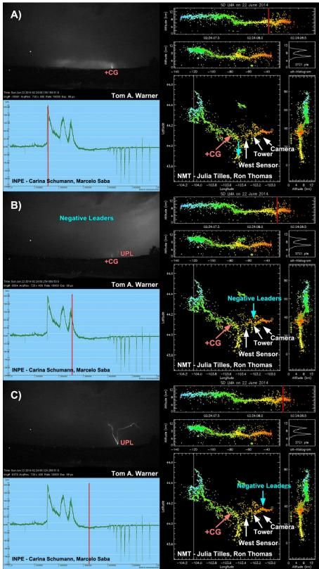
Figure 7 Composite figure showing images from a high-speed video recording (upper left panel), electric field change sensor recording (lower left panel) and LMA display (right panel). Red vertical lines show correlated time with high-speed video image.
