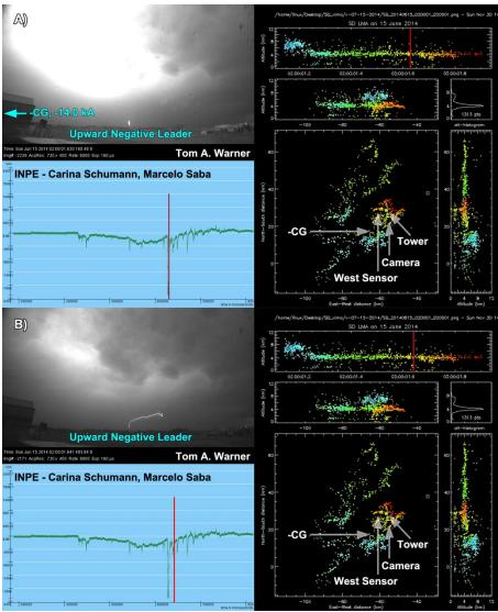
Figure 10. Composite figure showing images from a high-speed video recording (upper left panel), electric field change sensor recording (lower left panel) and LMA display (right panel). Red vertical lines in show correlated time with high-speed video image.
