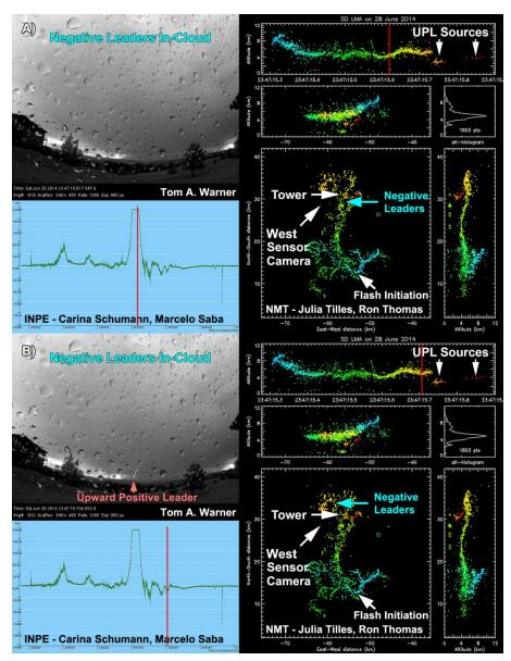
Figure 5. Composite figure showing images from a high-speed video recording (upper left panel), electric field change sensor recording (lower left panel) and LMA display (right panel). Red vertical lines show correlated time with high-speed video image.
