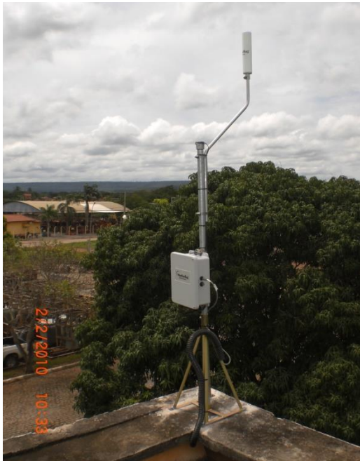
Fig. 9. Sensor to detect intracloud flashes from BrasilDAT.
