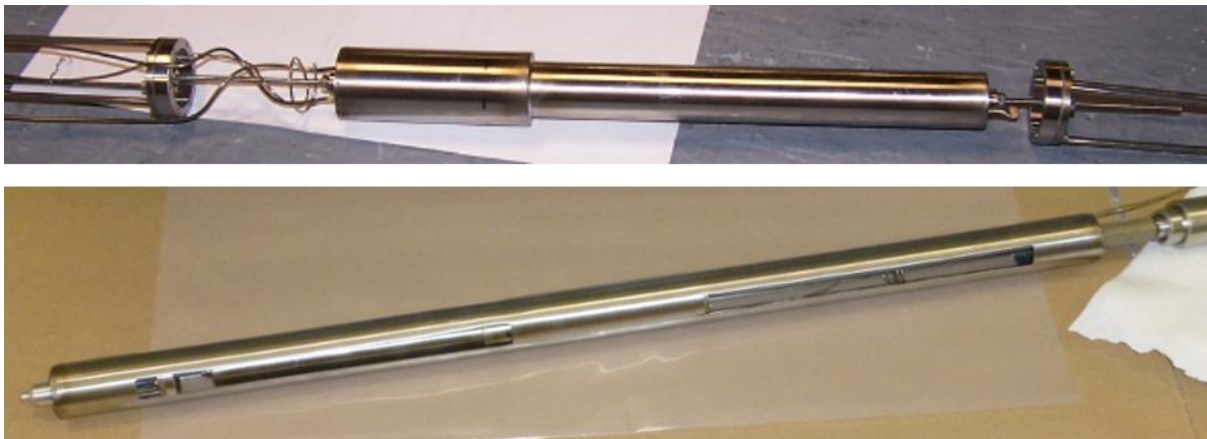
Figure 2. "Fuel rod" thermoacoustic sensor. (Above) The thermoacoustic resonator is shown at the center of the photograph. The resonator tube has an inside diameter of 2.2 cm and is 22 cm long. The insulated hot section of the resonator holds the hot heat exchanger that contains two enriched ^{235}\text{U} fuel pellets that are each approximately 5 mm in diameter and 10 mm long, as well as the extruded ceramic "stack" shown in Fig. 1. The resonator tube contains the 2.0 MPa He/Ar gas mixture. The empty portion of the resonator, to the right of the insulated section, is in good thermal contact with the reactor's coolant. Two 4-40 threaded rods extend from either end of the resonator. The rods are attached to two circular stainless steel disks (200 \mu\text{m} thick) that have six spokes acting as cantilever springs to allow the resonator to vibrate axially but constrain the resonator to remain coaxial within the surrounding "slotted tube." One of the thermocouples is silver-soldered (brazed) to the thin-walled section of the resonator next to the heat exchanger and the other is silver-soldered to the hot end of the resonator. Both thermocouples are located within the insulation space. (Below) The resonator and springs are contained within a "slotted tube" that has the same outer diameter as the fuel rods. The slots allow the reactor's coolant to remove the heat of fission from the thermoacoustic sensor and facilitated testing of the resonator's axial mobility before insertion in the reactor's core.
