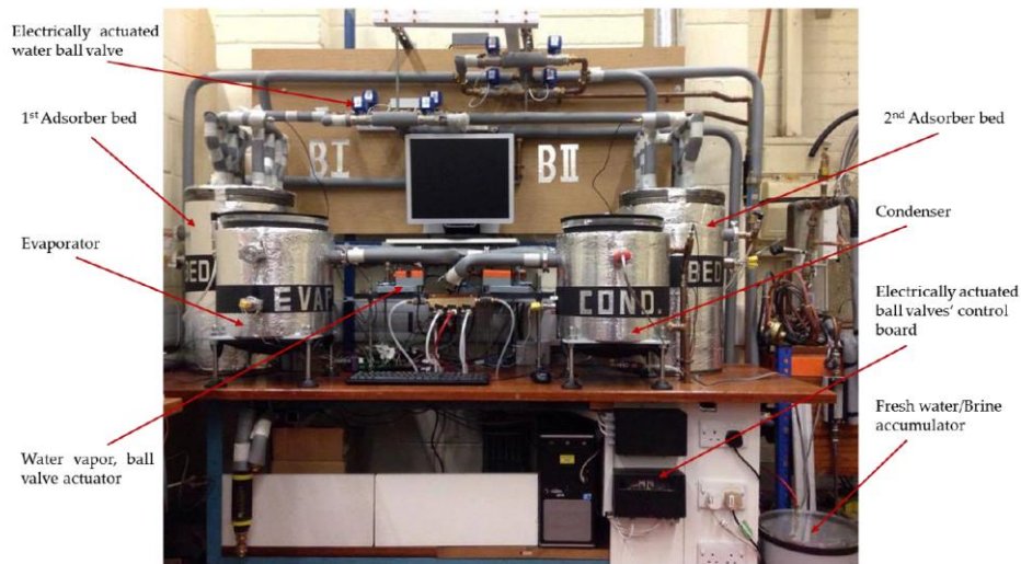
Figure 15, Testing facility of the double-bed adsorption system
