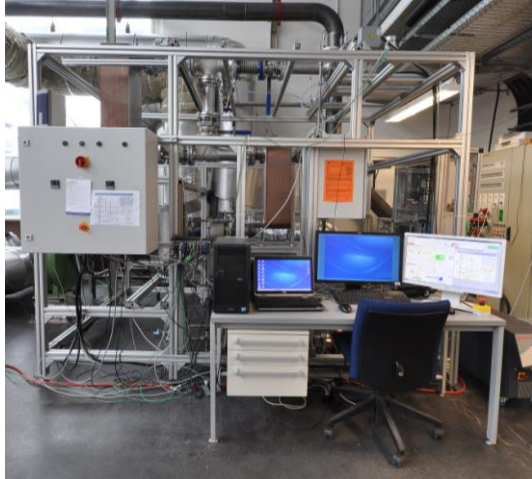
Figure 1: ORC test rig at the Center of Energy Technology with an electrical power of up to 15 kW
