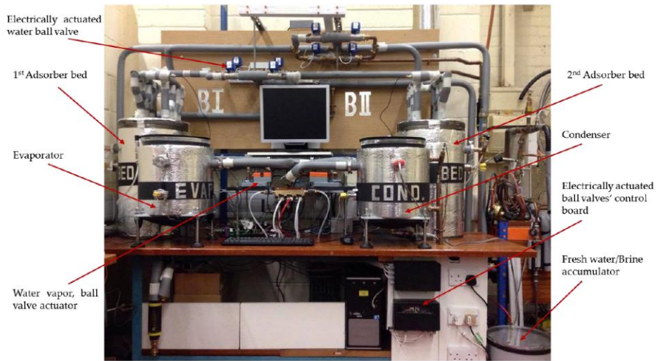
Figure 9, Testing facility of the double-bed adsorption system
