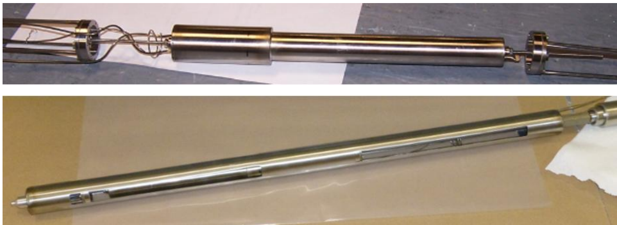
Figure 2. "Fuel rod" thermoacoustic sensor. (Above) The thermoacoustic resonator is shown at the center of the photograph. The resonator tube has an inside diameter of 2.2 cm and is 22 cm long. The insulated hot section of the resonator holds the hot heat exchanger that contains two enriched ^{235}\text{U} fuel pellets that are each approximately 5 mm in diameter and 10 mm long, as well as the extruded ceramic "stack" shown in Fig. 1. The resonator tube contains the 2.0 MPa He/Ar gas mixture. The empty portion of the resonator, to the right of the insulated section, is in good thermal contact with the reactor's coolant. Two 4-40 threaded rods extend from either end of the resonator. The rods are attached to two circular stainless steel disks (200 \mu\text{m} thick) that have six spokes acting as cantilever springs to allow the resonator to vibrate axially but constrain the resonator to remain coaxial within the surrounding "slotted tube." One of the thermocouples is silver-soldered (brazed) to the thin-walled section of the resonator next to the heat exchanger and the other is silver-soldered to the hot end of the resonator. Both thermocouples are located within the insulation space. (Below) The resonator and springs are contained within a "slotted tube" that has the same outer diameter as the fuel rods. The slots allow the reactor's coolant to remove the heat of
