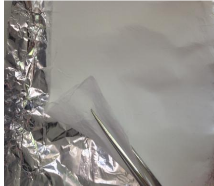
Figure 2. Fabric of silica gel microfibres deposited by electrospinning.
