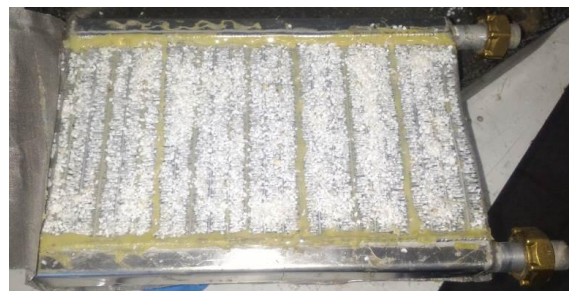
Figure 3: the heat exchanger filled with the composite material
