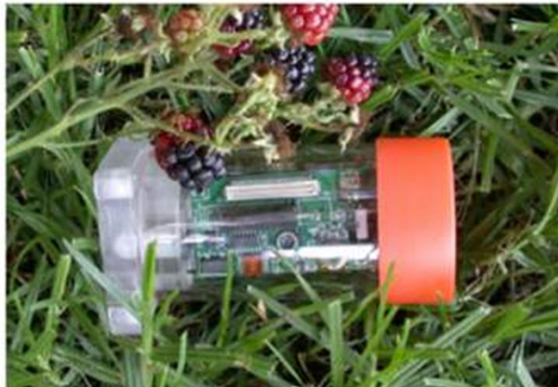
Figure 3: Acrylic enclosure used for deploying the Mica mote.
