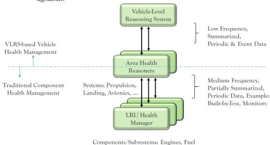
Figure 2.3 - Hierarchical view of component, area/system, and vehicle-level health management.
