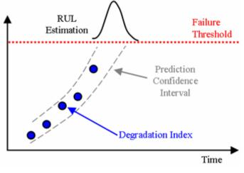
Figure 2.2 - Degradation index evolution and remaining useful life estimation.
