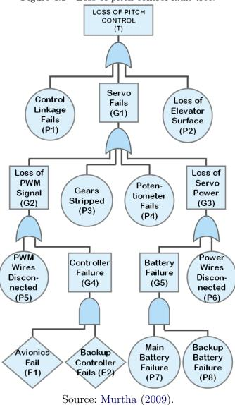
Figure 4.1 - Loss of pitch control fault tree.
