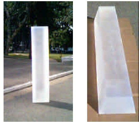
Figure 1: Plastic scintillators developed by IPEN to be used in the MASCO balloon-borne high energy imaging experiment.
