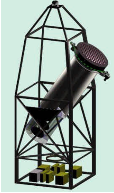
Figure 10: MASCO telescope in its flight configuration. The 7 meter high, 2 meter x 2 meter base, gondola will be suspended by a 1 million cubic meter balloon at 42 km of altitude.
