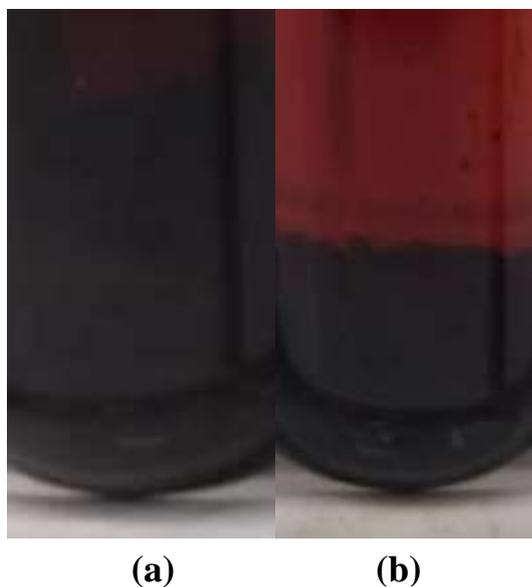
Figure 3. Bio-oil from sugarcane (a) without catalyst and (b) with catalyst.
