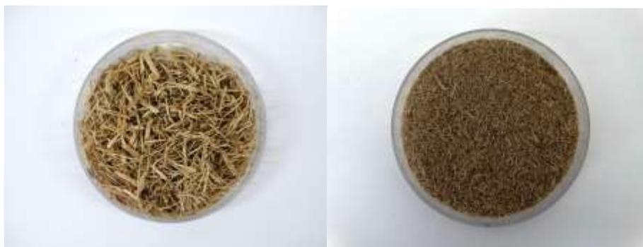
Figure 1. (a) Sugarcane bagasse (a) in natura; (b) particle size on range of 250 - 500 $\mu\text{m}$ .
