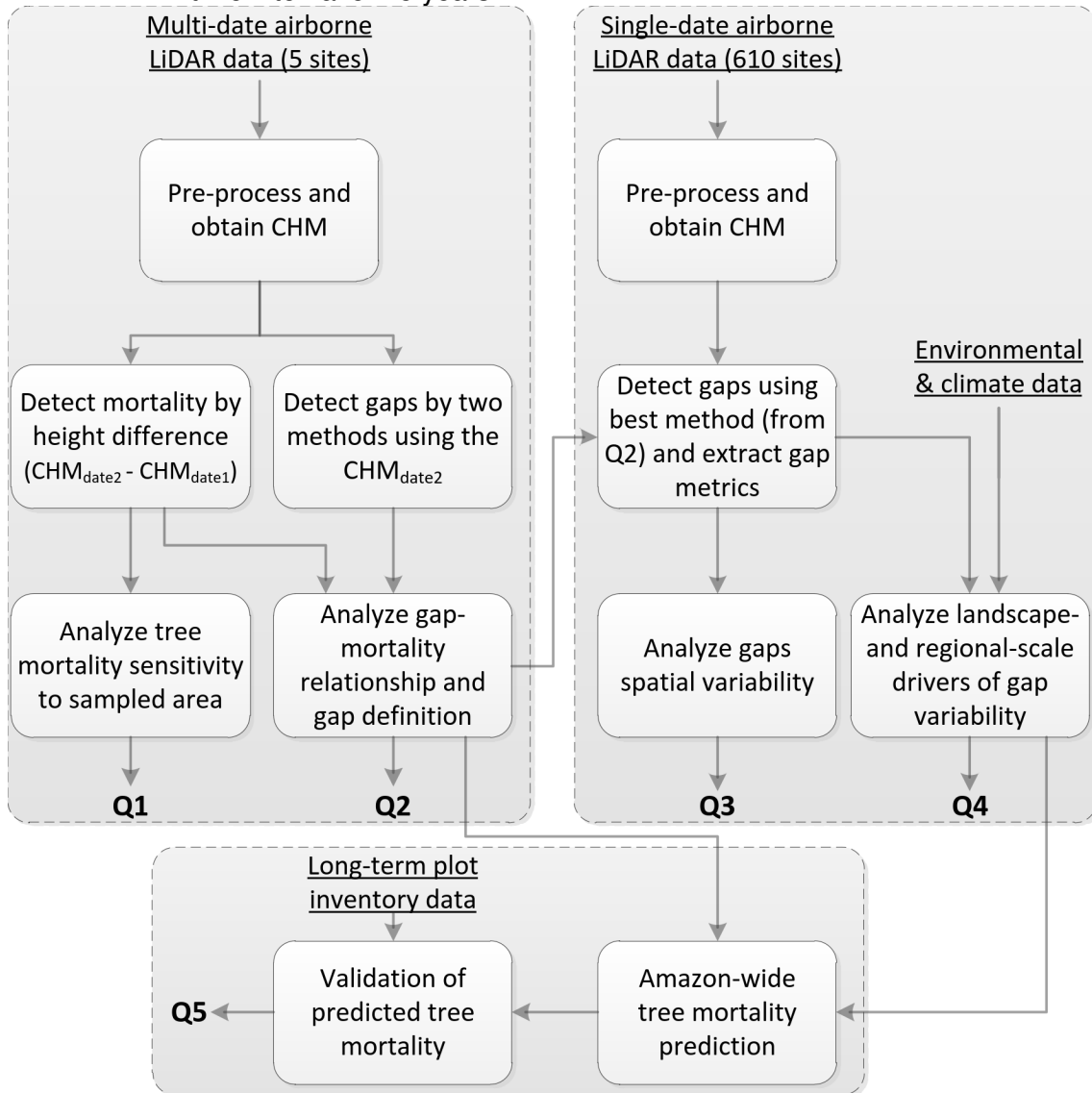
Figure 6.1 - Overview of the main methodological steps used to answer the research questions (Q1 to Q5). CHM date1 and CHM date2 correspond to canopy height models derived from LiDAR data acquired on two different dates with a time interval of ~5 years.
