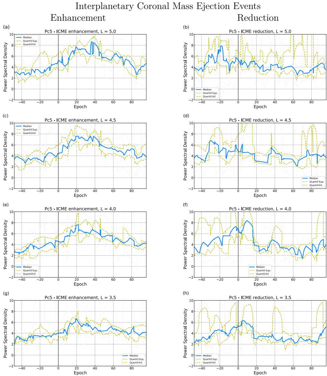
Figure 6.8 - Superposed Epoch Analysis Pc5 Power Spectral Density in L-shell values from 3.5 to 5.0 during flux enhancements (panels a, c, e, and g) and reduction (panels b, d, f and h), for ICME events. The solid blue line correspond to the median, while the yellow ones are the upper and lower quartile.
