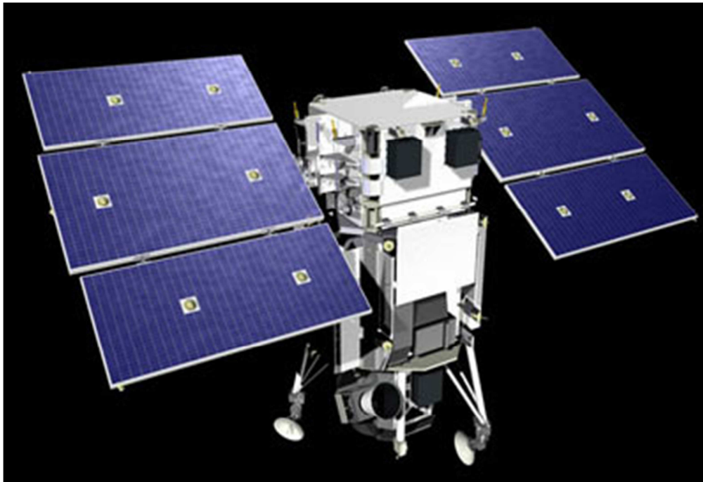
Figura 1.1 - BCP 5000 (WorldView 1) equipado com CMG de 1 cardan.
