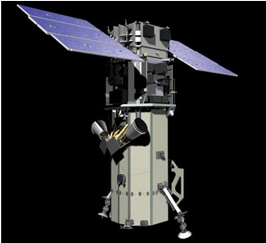
Figura 1.2 - BCP 5000 (WorldView 2) equipado com CMG de 1 cardan.
