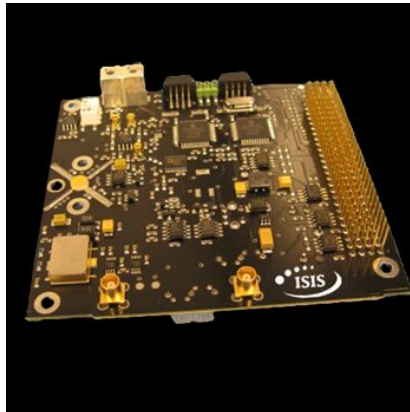
Figura 12: VHF downlink / UHF uplink transceiver – ISIS Space 12 .
