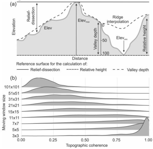
(a) Diagram representing the reference surfaces to derive the relative height, reliefdissection and valley depth (a). Elev = elevation; Elev<sub>max</sub> = maximum elevation; and Elev<sub>min</sub> = minimum elevation. (b) Effect of the size of the moving window in the derivation of topographic coherence, a scale-dependent variable. Note in b that there is a shift in the distributions, as the size of the moving window increases.
