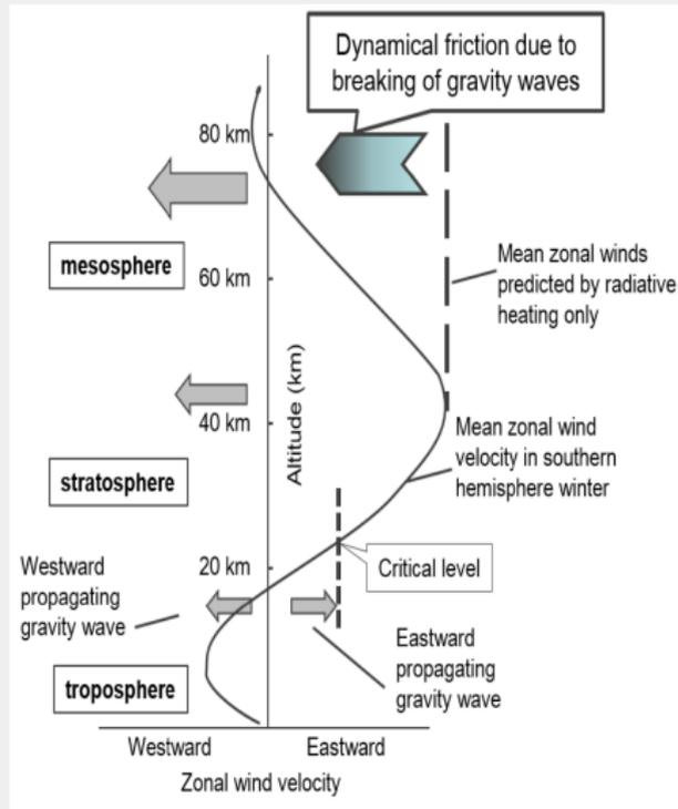
**Figure 4:** A schematic diagram depicting the fundamental concepts of interaction between mean winds and gravity waves [Tsuda, 2014].
