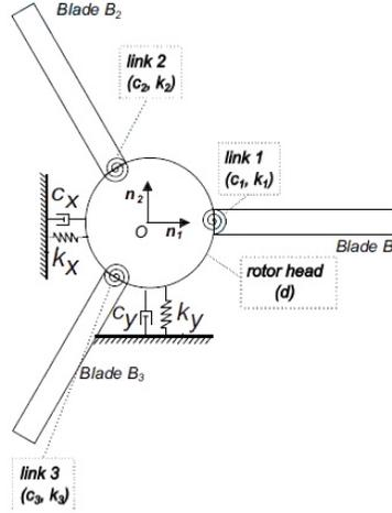
Figure 1: System Coordinate and Degrees of Freedom [6]
