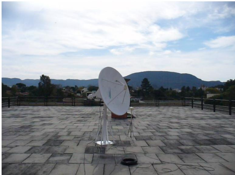
Figura 4.8 – Antena da *Professional HRPT SMART Station* Instalada para Testes no CRS/CCR/INPE
