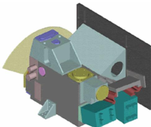
Fig. 4.4 – Esquema de montagem do Ozone Monitoring Instrument (OMI). Fonte: [http://aura.gsfc.nasa.gov/instruments/omi/omi\\_gallery.html](http://aura.gsfc.nasa.gov/instruments/omi/omi_gallery.html)
