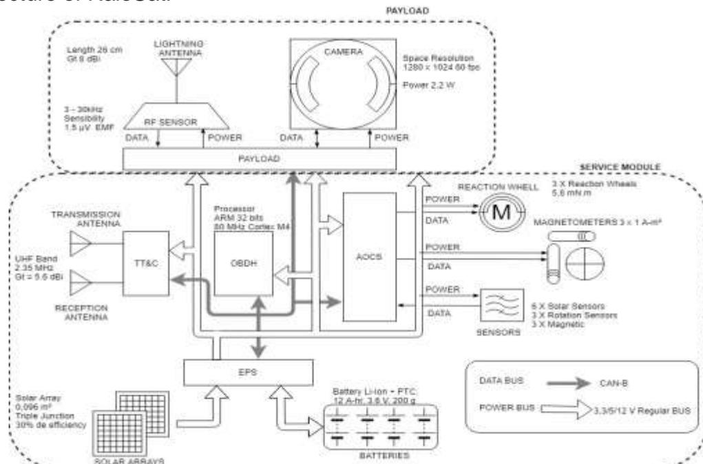
Figure 5: An instantiated physical architecture for RaioSat.
