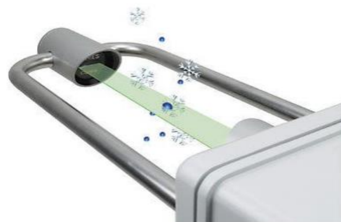
Figure 2 -Representation of droplets and ice crystals on the disdrometer sensor.
