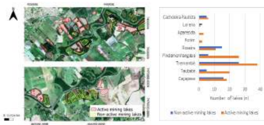
Figure 4. Classification of mining lakes (left) and quantity of non-active and active mining lakes (right).
