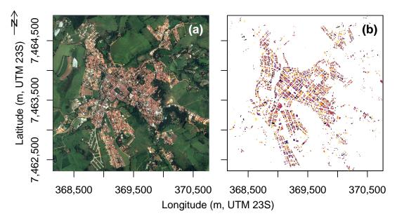
**Figure 7.** Main extension of Joanópolis (**a**) and the predicted instance mask of buildings (**b**). Satellite image courtesy of the DigitalGlobe Foundation.
