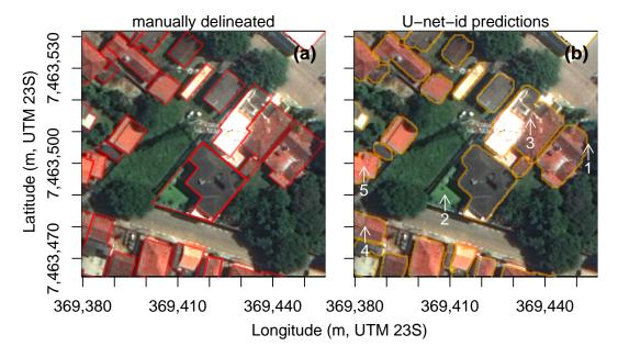
**Figure 6.** Example of a  $256 \times 256$  Joanópolis RGB image with the manually delineated (a) and the predicted instance mask of buildings (b). This subset of the image has been selected because it contains several of the main errors of the algorithm or of the producer (highlighted by the white arrows). Satellite image courtesy of the DigitalGlobe Foundation.
