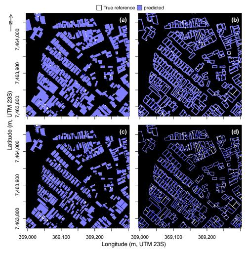
**Figure 4.** Example of the reference masks (in white) and predicted masks (in transparent blue) for: the segments (a); the borders (b); and the inner segments (c). The comparison between the reference building polygons and the predicted polygons generated by adding a buffer of 2 pixels around the polygon of the predicted inner mask is shown in (d).
