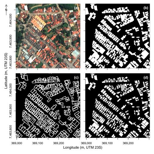
**Figure 3.** Example of a subset of the Joanópolis RGB image (**a**); and the corresponding masks for: building segments (**b**); borders (**c**); and inner segments (**d**). Satellite image courtesy of the DigitalGlobe Foundation.
