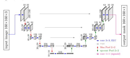
**Figure 2.** U-net model unit with characteristics of layer and filter sizes used in our model. The three U-net units used in our model are identical.
