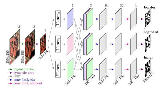
**Figure 1.** U-net-id model architecture. The three U-net units used in our model are identical but the three outputs of the U-net are represented with three different colors: magenta (U-net<sub>1</sub>), blue (U-net<sub>2</sub>), and green (U-net<sub>3</sub>).
