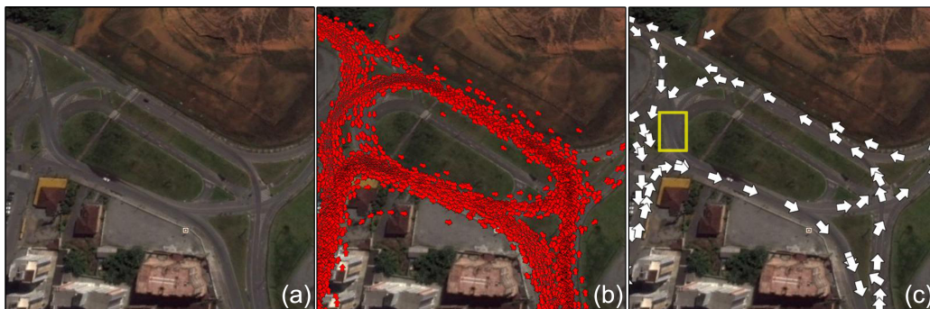
Figure 2. Second test: (a) satellite image; (b) points after preprocessing; (c) road centerlines with incorrectly mapped area highlighted
