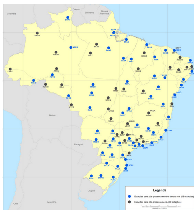
Figure 4. Stations configuration of RBMC. Blue points: real time stations; black points: post-processed stations. Image from IBGE website, available at < http://www.ibge.gov.br/home/geociencias/geodesia/rbmc/rbmc_est.php >.
