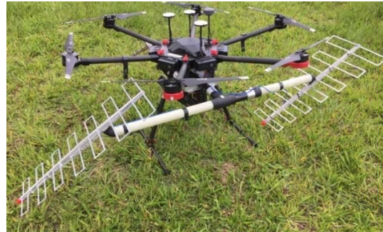
Fig. 2. P-band log-periodic antennas mounted on the drone.
