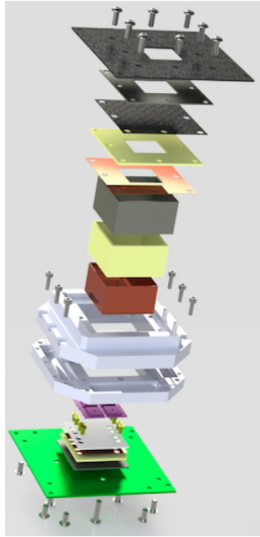
Figure 3. Exploded view of the LECX detector system. From top to bottom, the carbon fibre sheets, the shielding layers and box walls (Pb-Sn-Cu), the Teflon structure (two parts), the detector plane, the bottom shielding layers, and the cubesat PCB.
