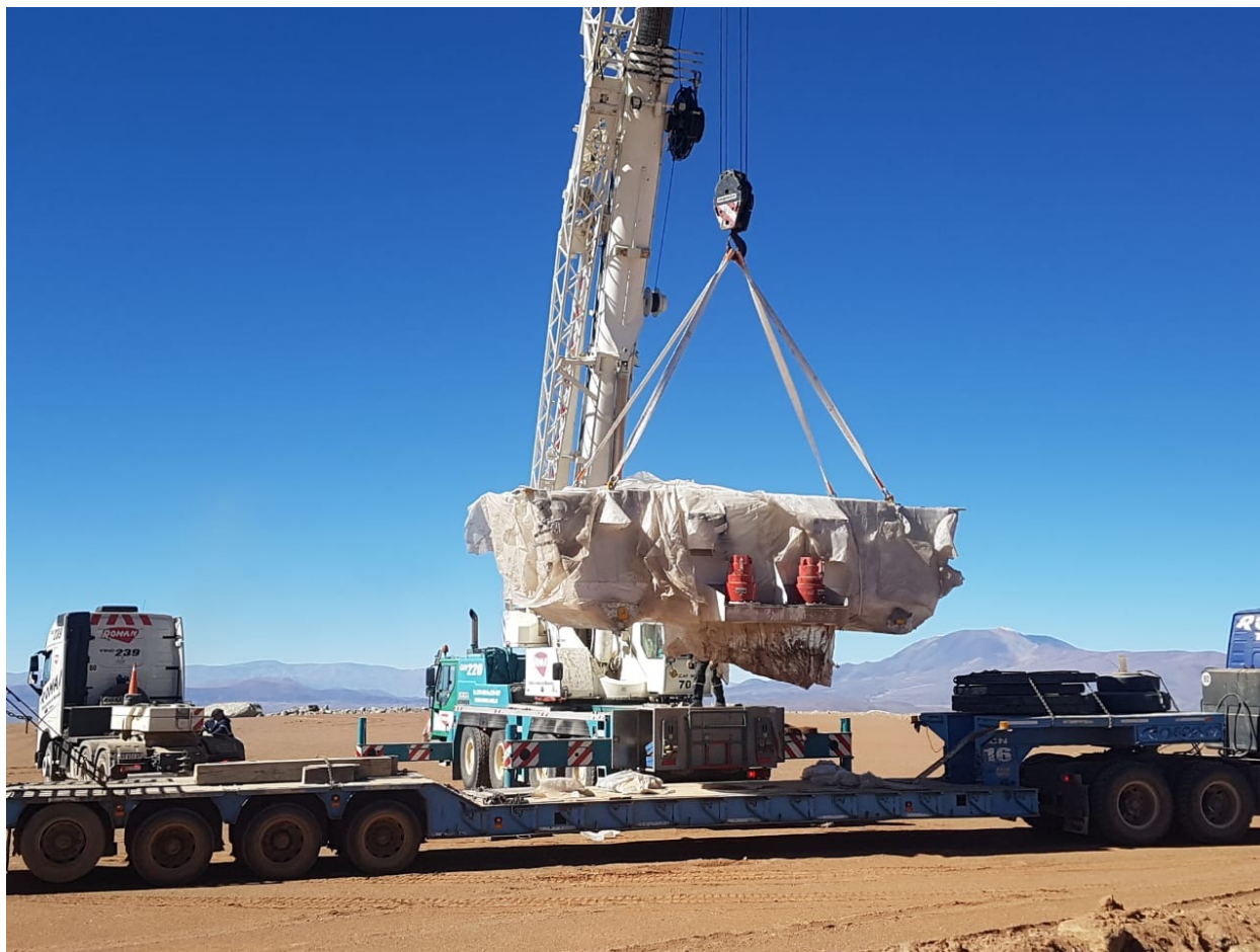
Figure 2. The Yoke Traverse, a piece of the antenna which had to be reconstructed by VERTEX due to an accident, arriving at the site of the observatory.
