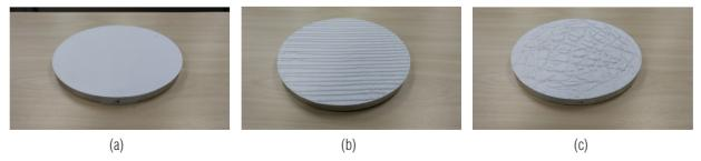
Figure 2 – Plaster surfaces used in the experiment. a) S1, flat and silky; b) S2, with nearly parallel grooves; c) S3, with random grooves.
