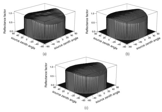
**Figure 6** – Reflectance Factor of the surface S2, with source ring fixed at azimuth angle  $\phi = 240^{\circ}$ . (a) 1°, (b) 8° and (c) 25° FOV.
