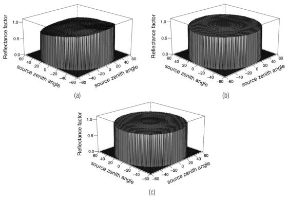
Figure 7 – Reflectance factor of the surface S3 at 850 nm, using (a) 1°, (b) 8° and (c) 25° FOV.
