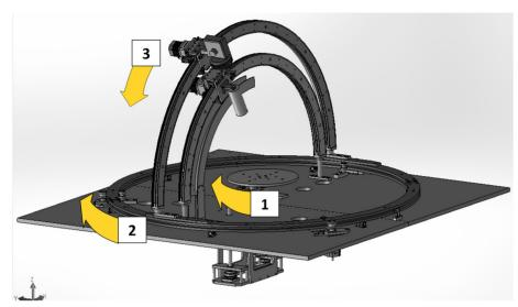
Figure 4 – Sequence of movements for the characterization of BRDF.
