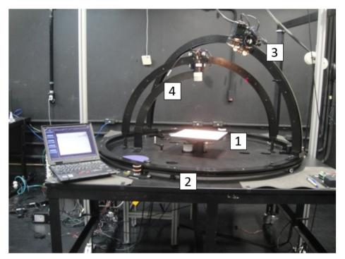
Figure 3 – Goniometer utilized during the in-lab BRDF determination.
