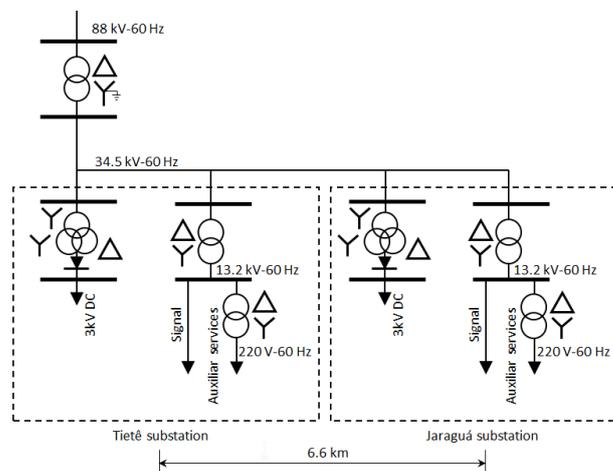
Figure 2. Schematics of the substations of Line 7.
