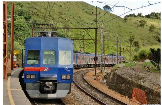
Figure 4. Train that runs below the transmission line and is powered by a 3 kV DC line.
