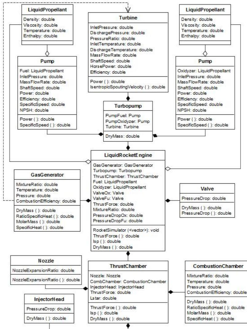
Figure 1. UML diagram of a gas generator cycle.
