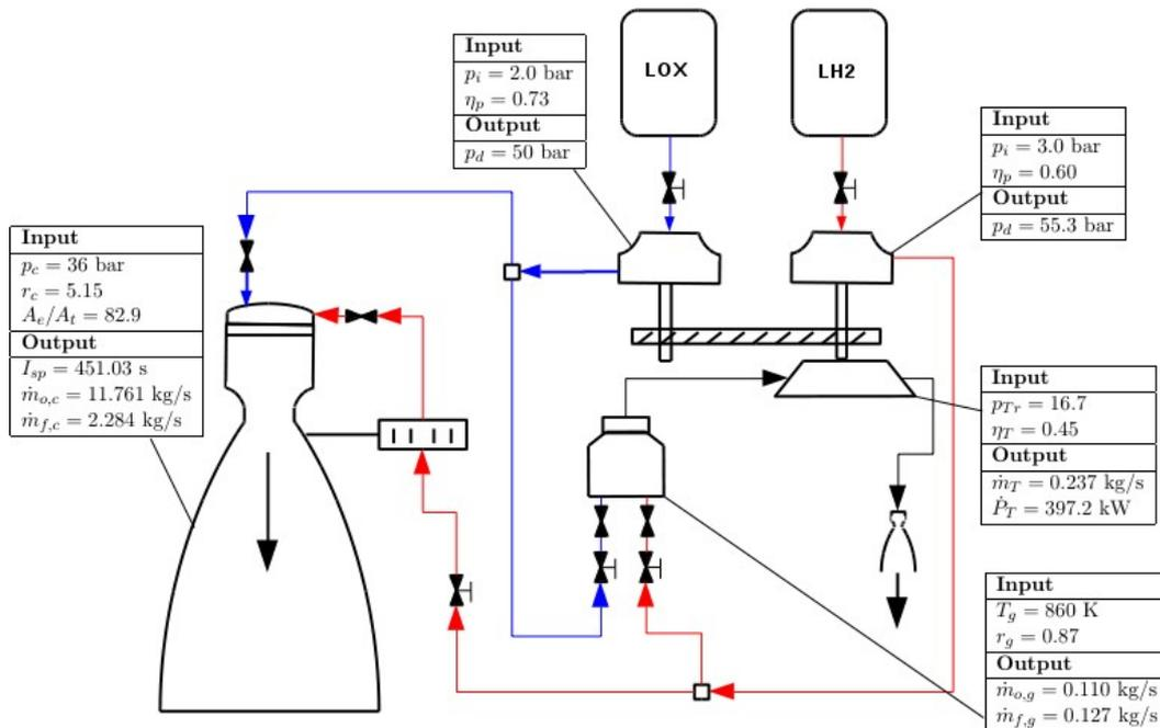
**Figure 3.** HM7B input/output (input data from Mc Hugh 1995).
