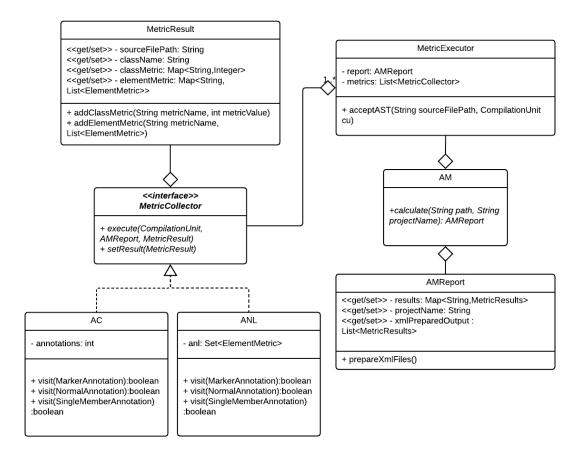
Figure 2. ASniffer Class Diagram.
