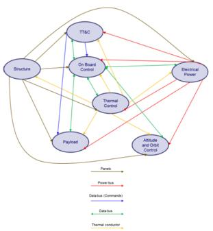
Fig. 32. Architecture interconnect diagram for product
