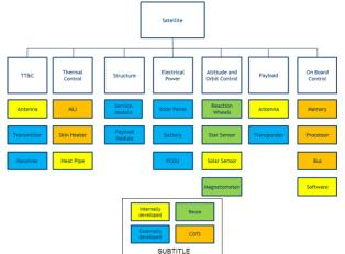
Fig. 34. Product Breakdown Structure (PBS)
