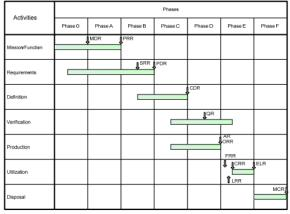
Phase 0: Mission analysis/needs identification Phase A: Feasibility Phase B: Preliminary Definition Phase C: Detailed Definition Phase D: Qualification and Production Phase E: Utilization Phase F: Disposal
