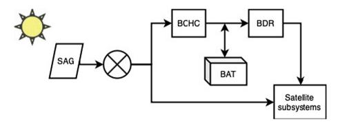
Fig. 2. Satellite power supply system block diagram
