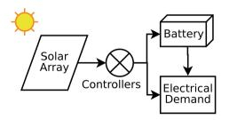
Fig. 1. Standalone photovoltaic power system
